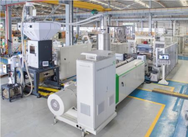
The extruder and roll stack technology can be used for in-line and out-of-line applications.
