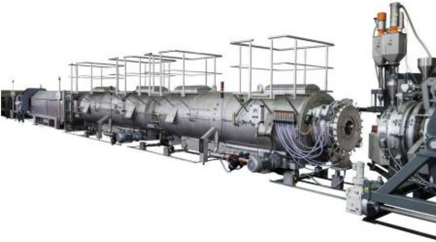
The FDC (fast dimension change) system enables pipe dimension changes during production
