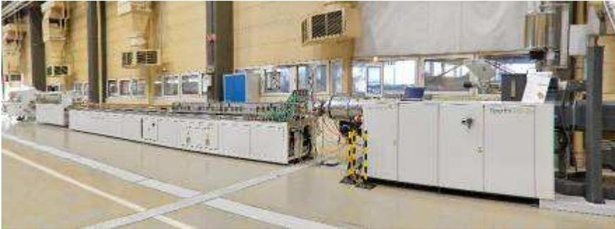
The extrusion line with the fiberEX 93-34D extruder, on which an H profile was produced
