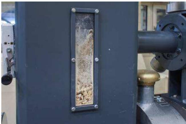
The agglomerate was compounded cost-efficiently in a heating/cooling mixer system; it was subsequently fed into the extruder without a dosing unit, simply by using the hydrostatic pressure of the material (shown in the picture: material feeding unit in operation, half-filled with WPC agglomerate)
