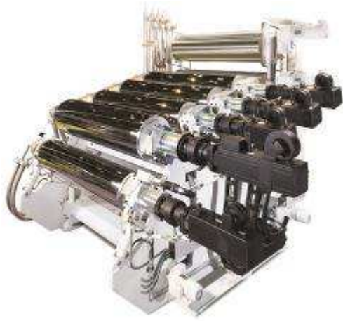
The Multi-Touch roll stack in XXL version – this model achieves outputs of up to 3,300 kg/h (PET)
