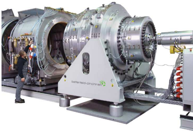
battenfeld-cincinnati offers complete large diameter pipe lines up to diameters of 2.6 m (PO) and 1.6 m (PVC)
