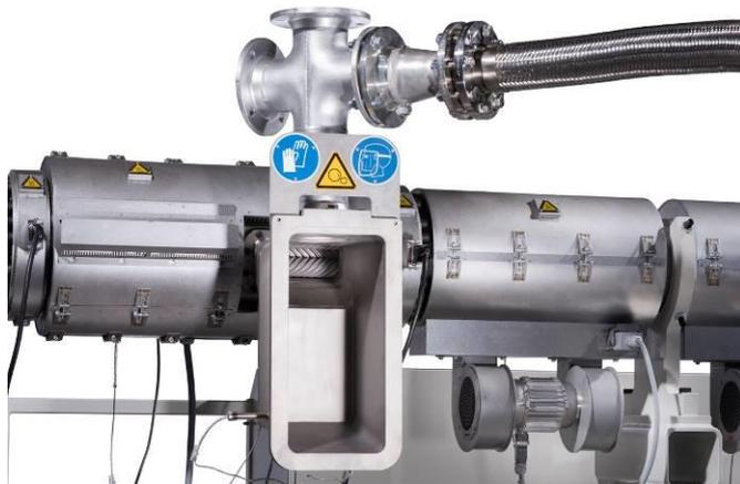
Close-up view of the planetary roller zone that ensures highly efficient degassing of the melt
