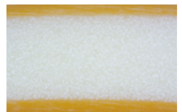
Enlarged view of the foam layer of a 3-layer PVC pipe
